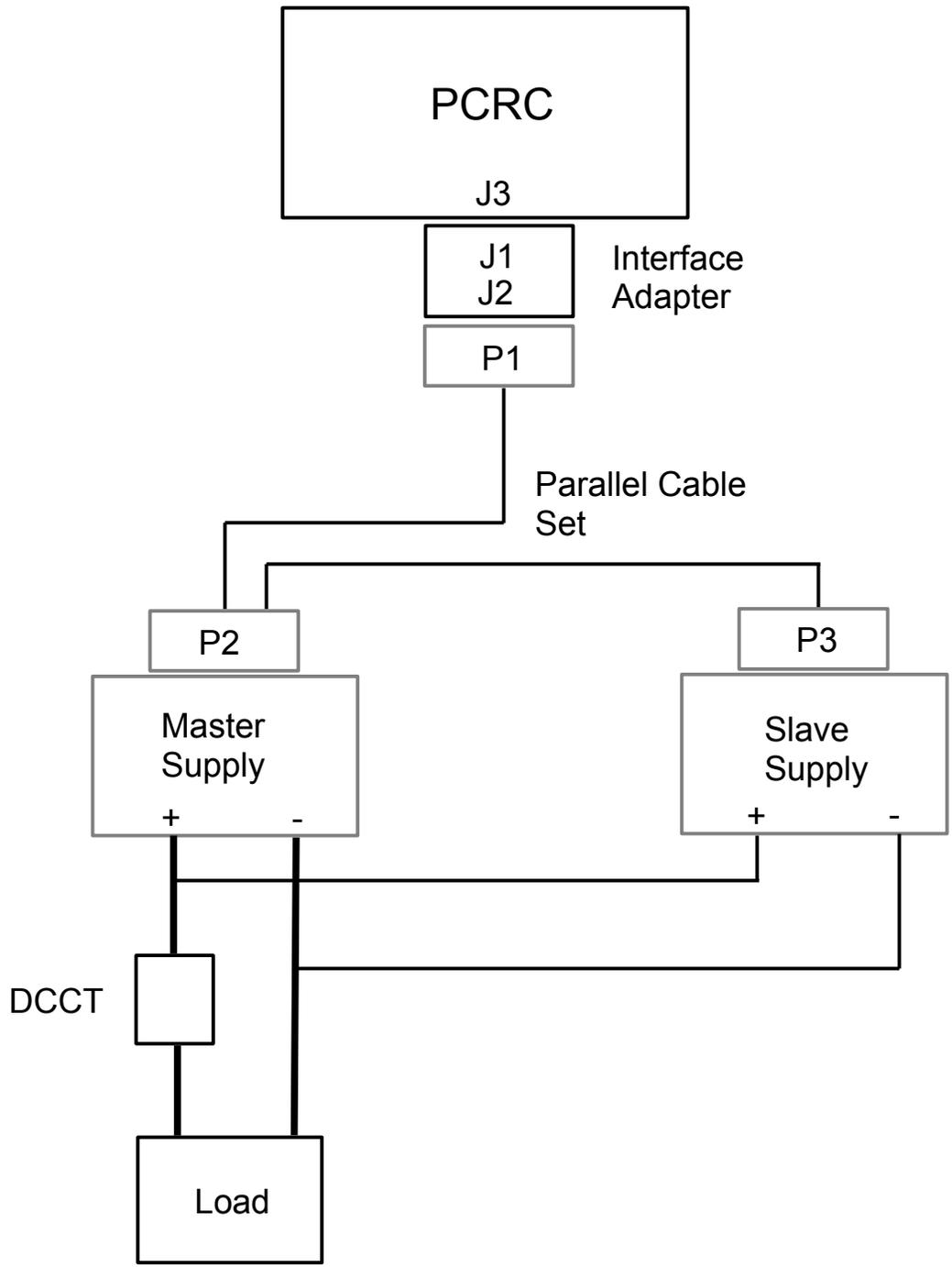
*Figure 10- Parallel Setup Configuration Diagram*
