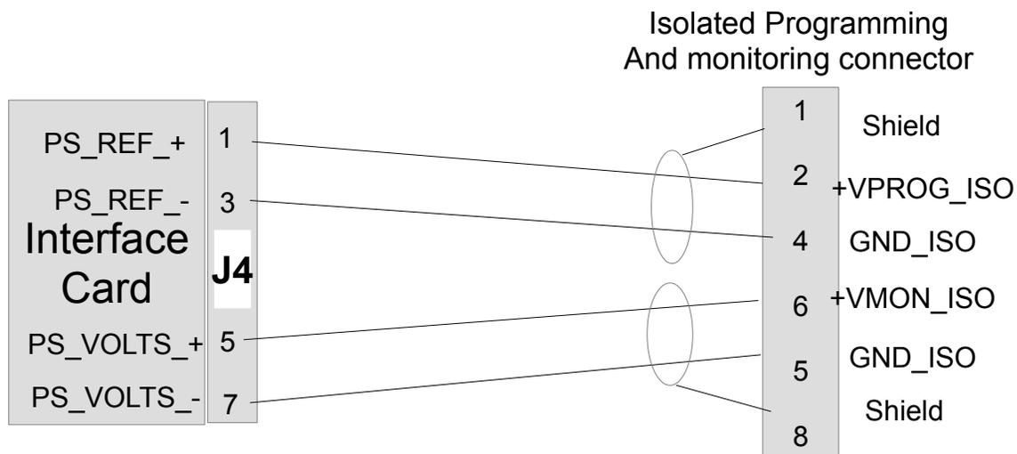
**Figure 7-** Isolated Analog Connections
